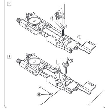
The size of a buttonhole is automatically set by placing a button in the rear of automatic buttonhole foot R.
