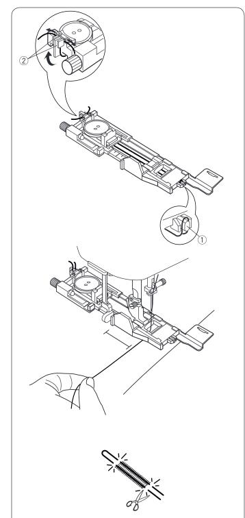
Place the button on the button holder on the buttonhole foot.
