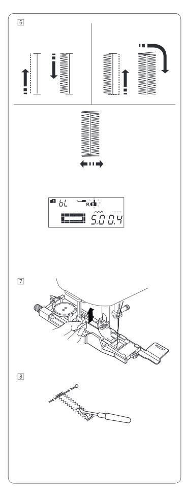
6 The buttonhole is sewn automatically in the sequence shown. When the buttonhole is nished, the machine will stop automatically with the needle in the up position.
