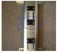
To adjust plastic holder move up / down by using screwdriver.
