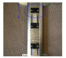
To adjust plastic holder move up / down by using screwdriver.
